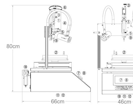
① Quickly adjust the angle of the oil delivery system to accommodate any cartridge form factor
